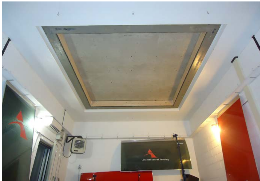
Receive Room View of Test Specimen Installation
