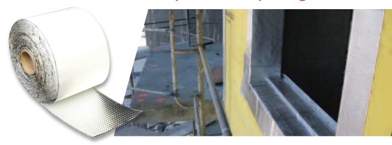
An All Purpose, Weatherproofing and UV Resistant Membrane for Skylights, Gutters, HVAC Units & Commercial Window Flashing **PROTECTO SEAL 45 BUTYL** is a cold applied, self-adhering membrane composed of a 45 mil high temperature recycled butyl adhesive, self-adhered waterproofing membrane with a tough cross laminated polyethylene film laminated to an aluminum foil for UV resistance and weatherability.
