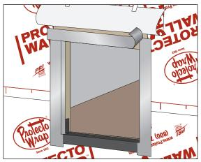
4. Apply PS45 Butyl Flashing with Protecto Spray Tak Primer at jambs with a minimum of 4" on the outer face of sheathing and a minimum of 2" into the rough opening. Do the same across the header and overlap the jamb flashings. Roll into place to ensure good adhesion.
