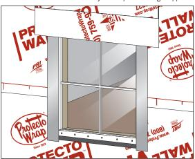
7. After the window has been flashed, un-tape the horizontal piece of Protecto Wall VP above the header, remove the release liner and fold down into position to cover over the header flashing. Roll the Protecto Wall VP into place to assure good adhesion. This completes the Flashing Installation.
