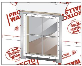
5. Apply Protecto Sealant 25XL to the back side of the window nailing fins at the jambs and header and install the window with fasteners. Remove any excess sealant from beyond the edges of the fins and allow residue to dry before post flashing is applied.
