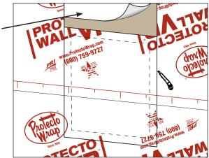
1. Cut the Protecto Wall VP 2" beyond the rough opening at the sill, jambs and a minimum of 6" above the header. Remove the Protecto Wall VP to expose the sheathing from the rough opening out to the cut lines.
