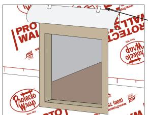
Apply additonal Protecto Wall VP above header flashing as needed in a shingling overlap fashion
