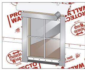
6. Post Flash over the window fins with PS45 Butyl Flashing with Protecto Spray Tak Primer at jambs and then across the header overlapping the jamb flashings. Roll to ensure good adhesion.
