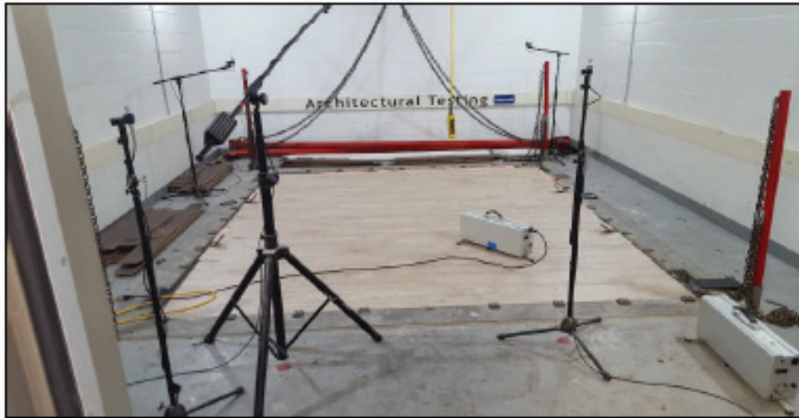
Source Room View of Test Specimen Installation
