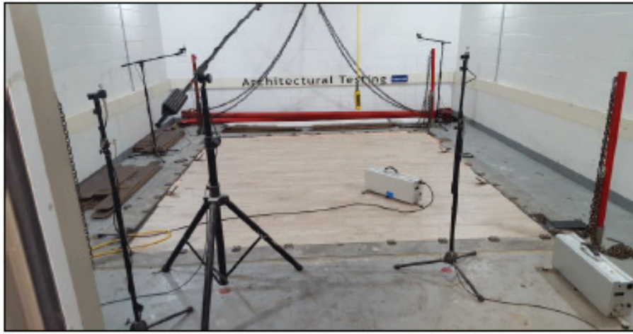
Source Room View of Test Specimen Installation
