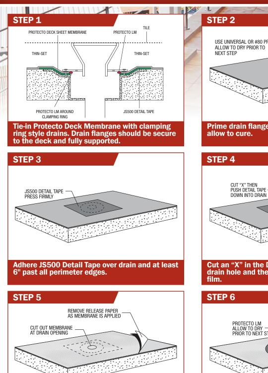
Apply the Protecto Deck Membrane and firmly press the Membrane to assure good adhesion to substrate and to Detail Tape.
