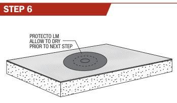
Apply Protecto LM to seal edge at the Drain Opening and 4" out onto the Membrane.
