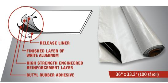
Protecto Roof is a self-adhered, exposable roofing and waterproofing membrane consisting of a reinforced white aluminum finished surface combined with a layer of high-quality butyl rubber adhesive. The flexibility of the membrane and the allows for ease of application to many configurations and various uses including low pitch applications typically found on garages, porches, manufactured housing, metal buildings or as flashing on skylights and vents.
