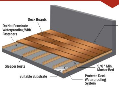
Restrain Finished Deck At Walls & Handrails To Prevent Vertical Movement/Uplift
