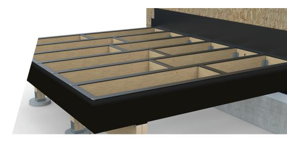
A self-adhering, cold-applied tape used as flashing on rim joists without the need for a primer
