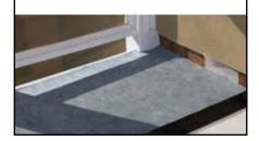
**6** Cut fabric to sit around all transitions, posts and protrusions.
